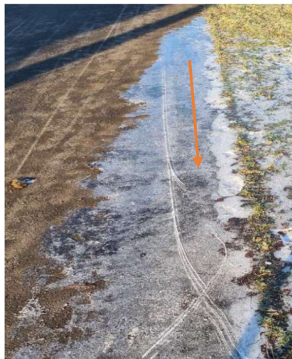
Figure 3: Examples of wheel tracks at 100% slip (hard braking) and slippery surfaces.
